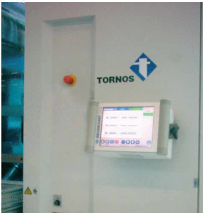
A BRANKAMP ET terminal with integrated in-process dimension measurement by Huber Systems on a Tornos Multideco. The multiple-spindle automatic lathe for mass production manufactures turned parts for the automobile industry.
